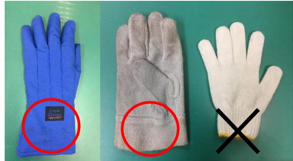
Fig. 2. 断熱手袋，革製手袋と軍手 Thermal insulating gloves, leather gloves and cotton work gloves
